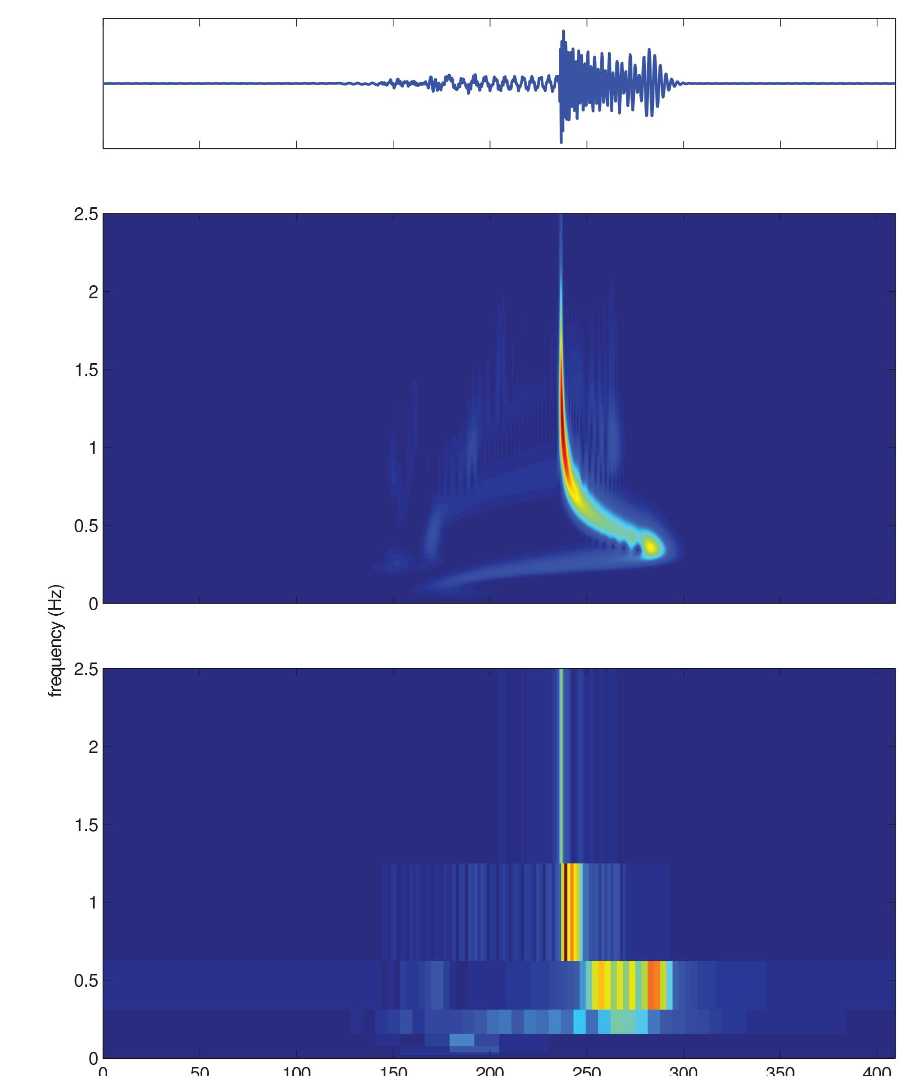
EXAMPLE OF A SYNTHETIC SEISMOGRAM (TOP) WITH THE ABSOLUTE VALUE OF ITS S-TRANSFORM (MIDDLE) AND THE COEFFICIENTS OF THE DOST BASIS VECTORS
