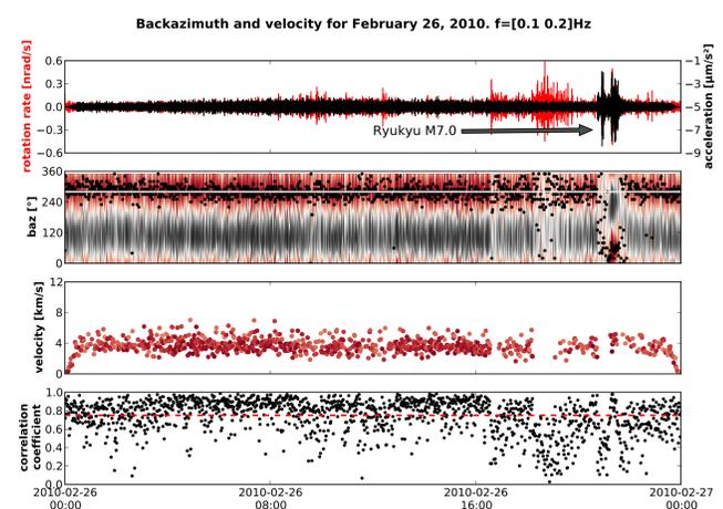
(a) Rotation rate (red), transverse acceleration (black). Event ( $M_w 7.0$  Ryukyu) with backazimuth =  $45^\circ$ . (b) Backazimuth, colorscale is the cross-correlation coefficient (red: positive high; black: negative high). (c) Phase velocity obtained from amplitude ratio ( $\frac{a_T}{\omega_z}$ ). (d) Maximum correlation coefficient.  $f = [0.1 \ 0.2]$ Hz
